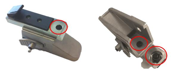
Images of listed Tire Changer Clamping Adaptors. Check circled fasteners for proper torque (16 lb-ft).
