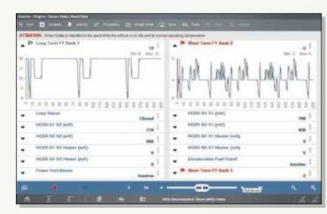
View filtered PID lists and graphs specific to the vehicle and fault code. Flags highlight data that is out of expected range.
