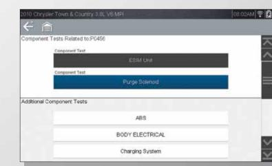
Built-in scope lets you verify component failure. Its guided Component Test Meter pinpoints fault codes at a glance, helping you quickly identify the faulty component.
