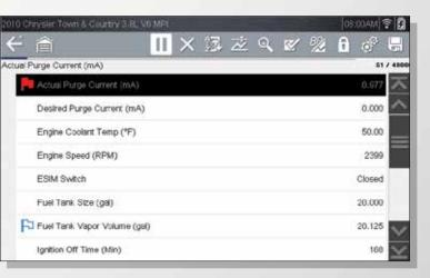
The smart choice for smart data. With built-in "Smart Data", TRITON-Dg automatically configures the display to show vehicle parameters (PIDs) relevant to the fault code. It saves you even more time by filtering out non-related data parameters.
