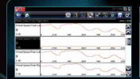
Consistent navigation for all OEMs. Digital and graphing display plus powerful scan tool functions to make the job easier: custom data lists, zoom view, min/max capture, triggers, record up to 2000 frame data movies.
