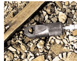
Easily removing rusty nuts during railroad construction is just one of many application examples for the Enerpac Nut Splitter.
