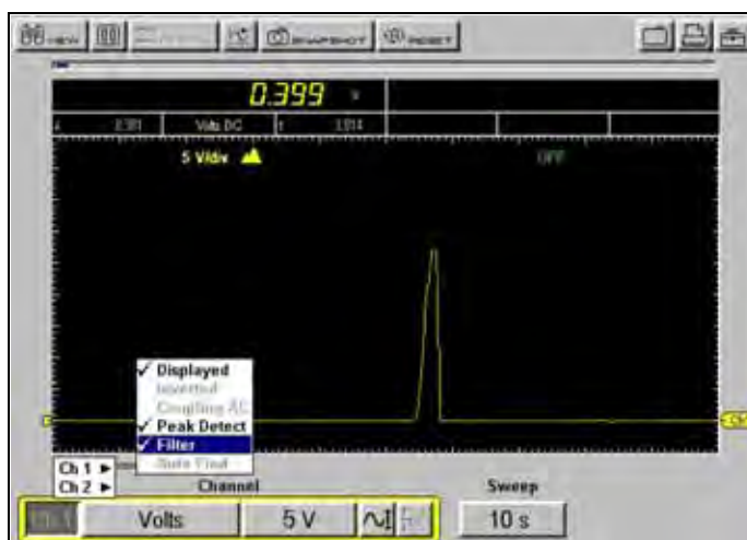
Figure C-6 Sample Noise Filter on—TPS Sweep (KOER)
