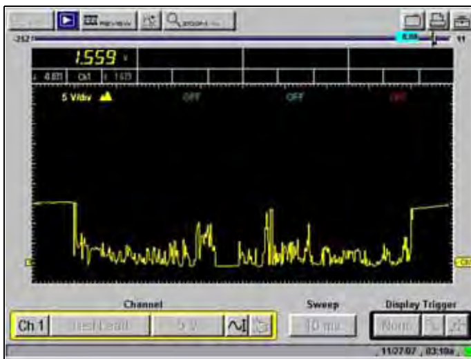
Figure B-6 Sample Faster Sweep—TPS Glitch captured
