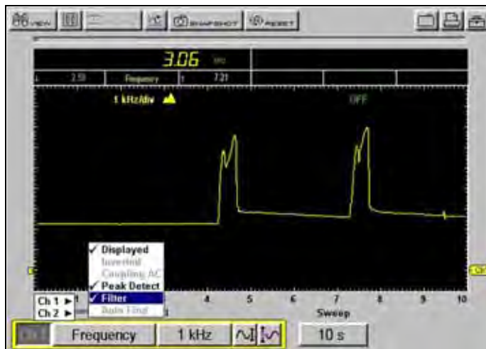
Figure C-2 Sample of Frequency with Filter on
