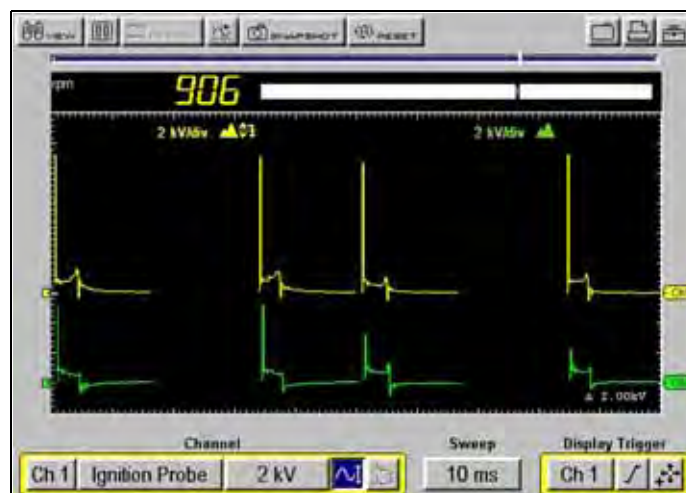
Figure D-9 Sample 6/3 coil not firing and not detected
