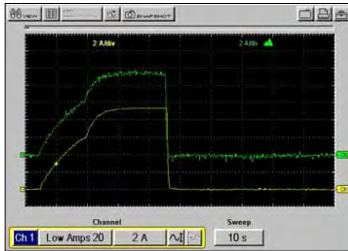
Figure C-7 Sample Noise Filter—two low amp scope probes
