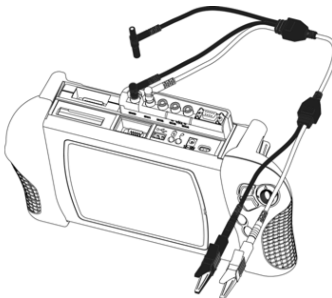
Figure 2-1 Sample yellow lead connection
