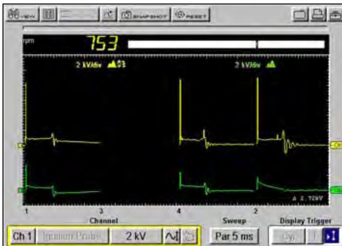
Figure D-7 Sample sensitivity set too high
