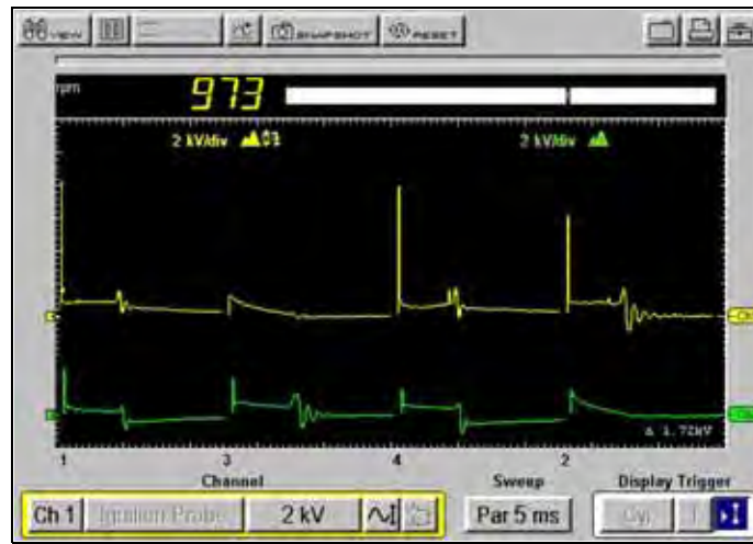
Figure D-8 Sample shorted spark-plug detected
