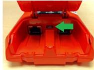
5. Connect the standard USB connector end of the USB cable to the display unit.
