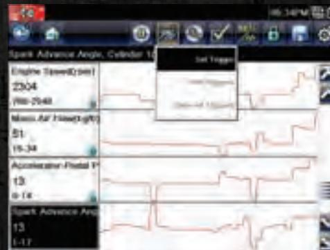
Display live data parameters digitally or graph from one to four on-screen at once. View detailed results over time and use powerful tools to find faults: triggers, zoom, record and playback movies and screen images.
