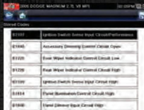
Read and clear OEM-specific codes and Global OBD-II Codes in seconds. See detailed code definitions on-screen.
