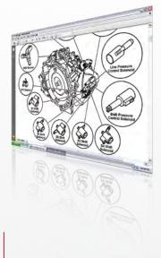
Touch any data PID to view it in text, graph or full-screen mode. View up to 16 live data graphs at once, to see true cause and effect.
