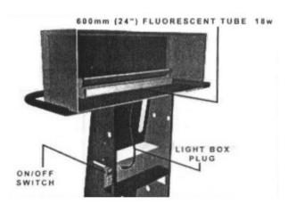
Installation of light box cable to IEC socket
