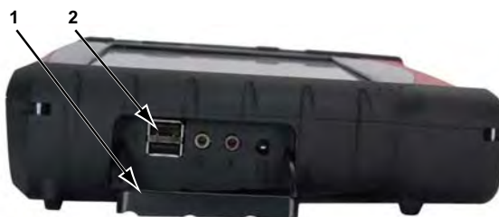
Figure 8-3 Scope Multimeter module USB jack location
