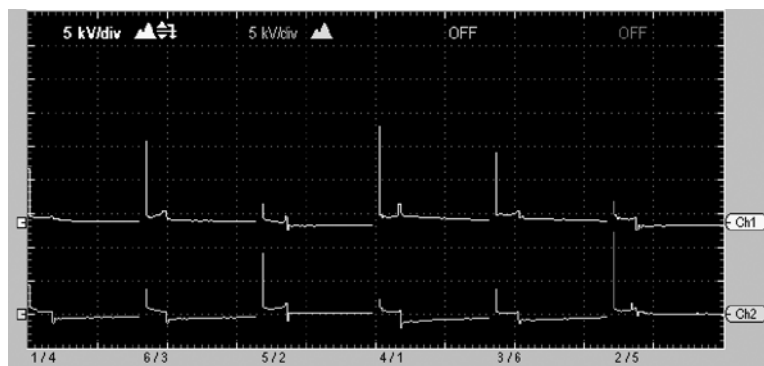
Figure 4-9 Incorrect polarity setup
