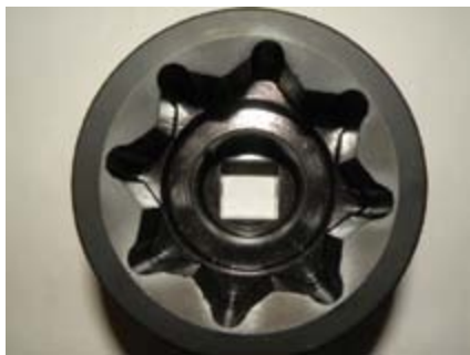
Above, a flank drive socket in action. The proper use of a flank drive in removing fasteners is key. Snap-on flank drive wrenches and sockets were developed to provide the proper amount of torque to remove the fastener, while not rounding off the corners.
