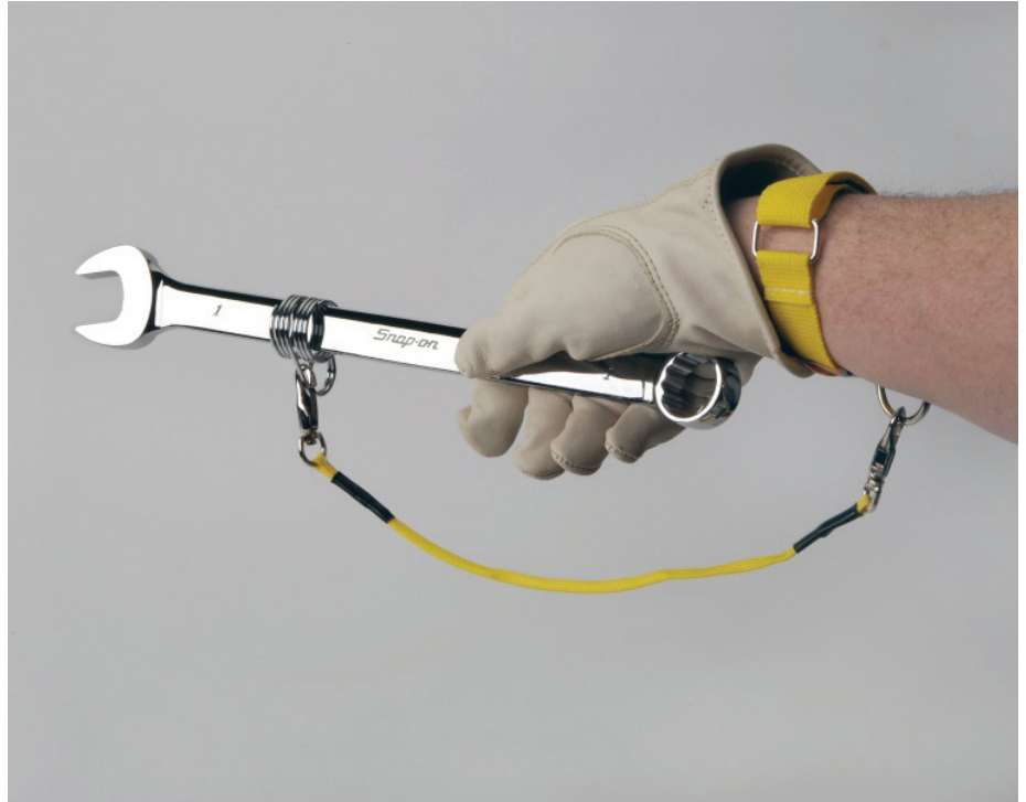
A robust system of tethering referred to as "Tools at Height" can help prevent injury and equipment damage due to droppage.
